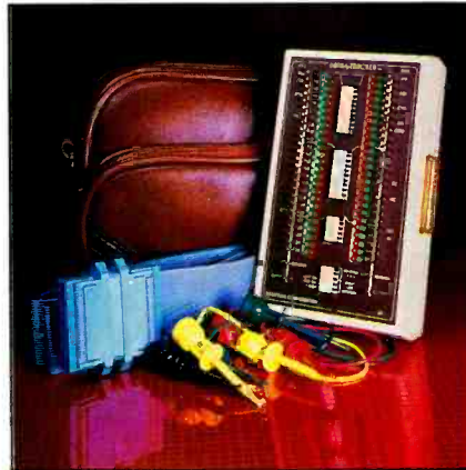
Page 52—A break-out box connected between a computer and a peripheral monitors the signals and helps determine the problem.
