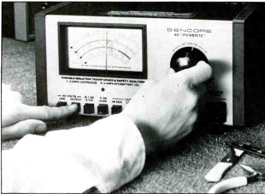
Figure 2. Use an adjustable, isolated ac power supply to reduce the voltage to the receiver. This gives you manual control of the voltage regulator, which lets you find what is causing the circuit problem.
